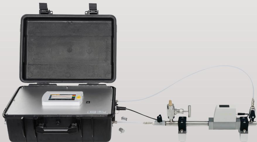
OMI-AR600 with the isokinetic sampler attached
