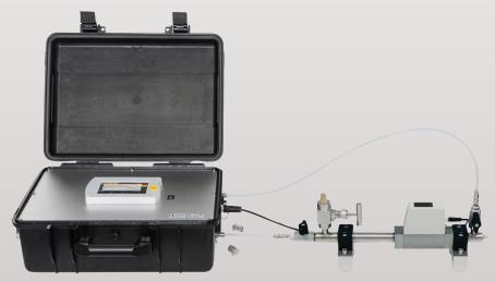
For particle measurements according to ISO 8573 an isokinetic sampling tube has been designed. This optional equipment enables you to monitor and adjust the air flow of the particle measurement to ensure the correct isokinetic sampling.
