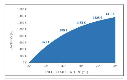
Savings based on the reduction of the inlet air temperature
