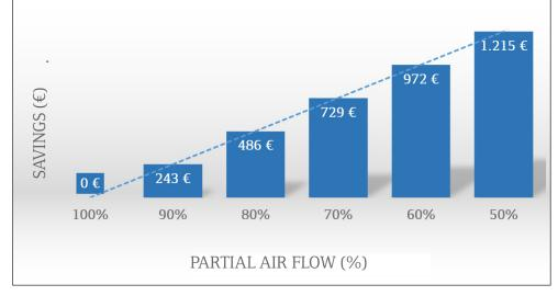
Savings based on a dryer working with a variable partial airflow half of the operating time (1000 hours)
