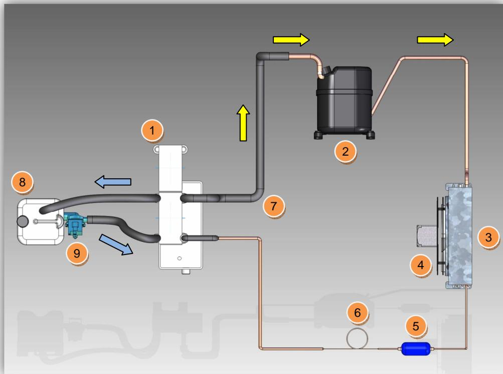
When operating at partial loads, the dryer can exploit the energy previously stored in the glycol circuit to shut down the compressor and substantially save energy and costs.
